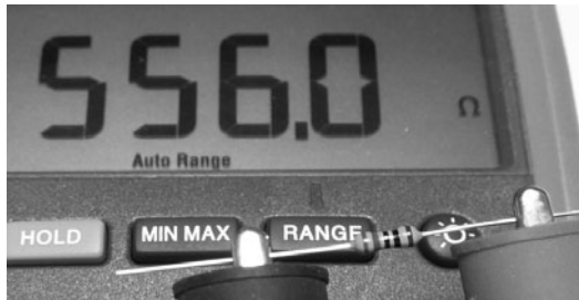
Figure 3-4: Multimeter measuring a 560-ohm 1 percent tolerance resistor
