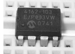
Figure 17-11: Microchip Technology's MCP4162 digital rheostat
