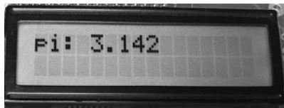
Figure 7-4: LCD displaying a floating-point number
