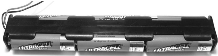
Figure 12-11: Battery holder with six AA cells
