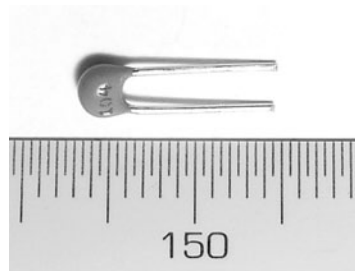
Figure 4-12: A 0.1 \mu F ceramic capacitor
