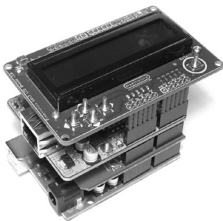
Figure 8-4: Three stacked shields with an Arduino Uno
