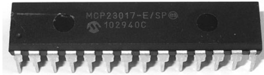
Figure 17-5: Microchip Technology's MCP23017 port expander IC
