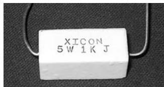
Figure 3-5: A 5-watt resistor
