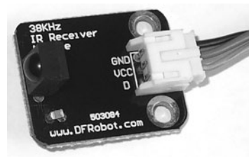
Figure 15-2: Prewired IR receiver module
