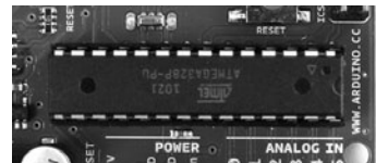
Figure 11-13: Correct orientation of the microcontroller in an Arduino
