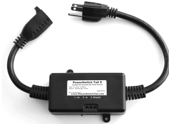
Figure 4-42: A PowerSwitch Tail that switches up to 120 V AC
