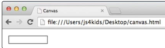
Figure 13-4: Using strokeRect to draw the outline of a rectangle
