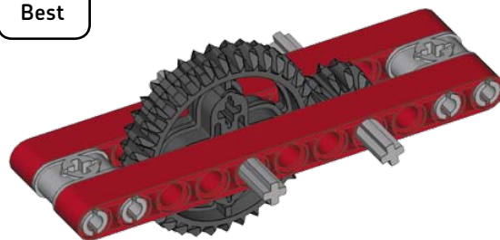
Figure 11-23: Bracing gears with beams ensures that their teeth do not slip.
