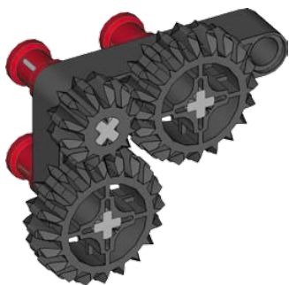
Figure 11-14: Creating a gear train along the corner of a beam. Both 20T gears turn in the same direction and at the same speed. The 12T idler gear has no effect on the gear ratio.
