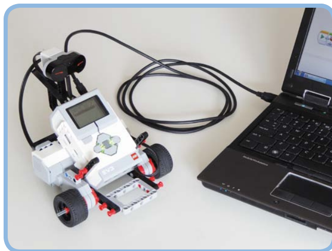
Figure 3-1: The robot connected to the computer using the set's USB cable. Use the USB connection at the top of the EV3, as shown here.
