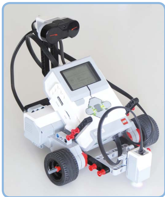
Figure 7-1: Using the Color Sensor, the EXPLOR3R can detect colors and follow lines.
