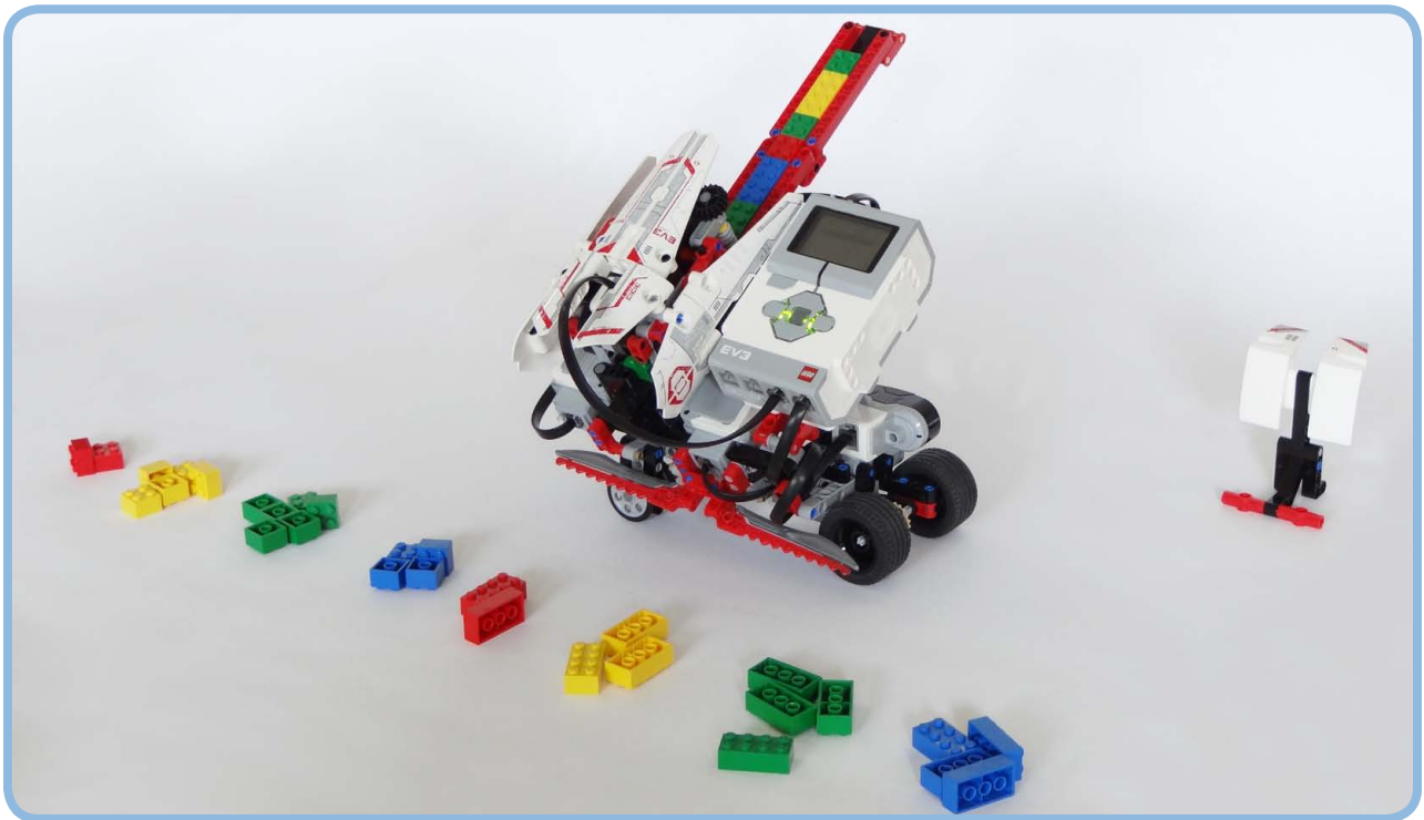
Figure 19-21: Feel like building another robot? The BRICK SORT3R sorts LEGO bricks by color (red, yellow, green, and blue) and size (2x2 and 2x4). You can find building and programming instructions at the book's companion website.
