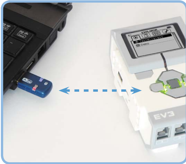
Figure A-12: One setup for wireless programming with Bluetooth
