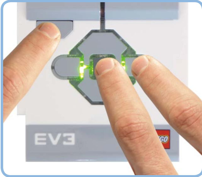
Figure A-10: To put the EV3 in Update mode manually, hold the Back, Center, and Right buttons until the brick status light turns off. Then, release only the Back button. Once the screen reads “Updating..”, release the other buttons.
