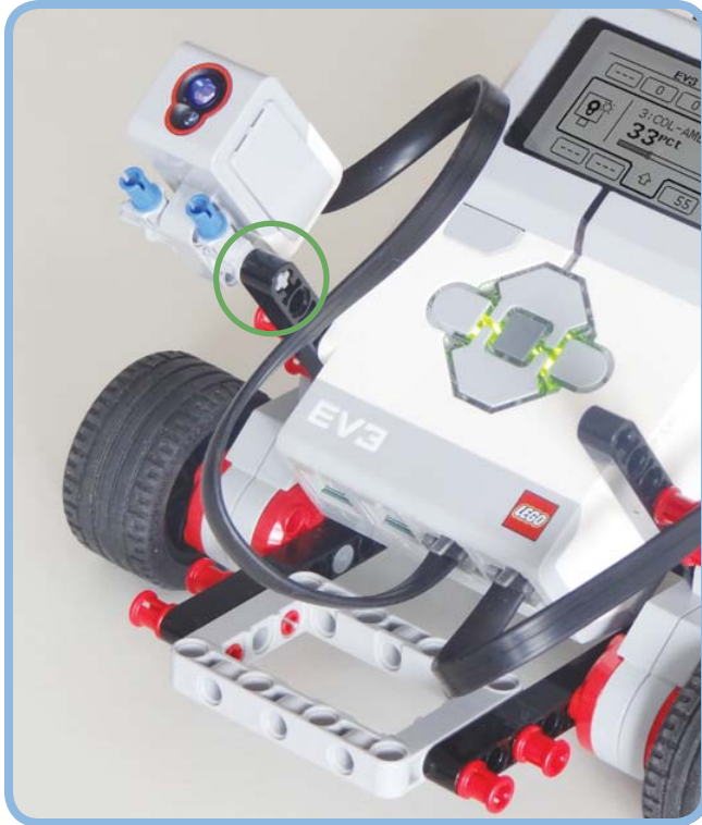
Figure 7-16: Remove the Color Sensor from the front of your robot and reattach it to the side. You won't need any additional LEGO elements. The cable remains connected to input port 3.
