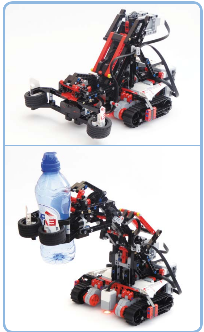
Figure 18-1: The SNATCH3R can grab and lift lightweight objects, such as empty water bottles.
