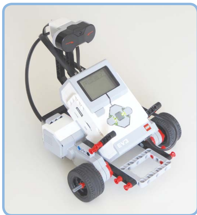
Figure 2-1: The EXPLOR3R moves around on two front wheels and a support wheel in the back.
