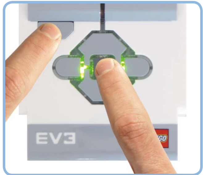
Figure A-9: To restart the EV3, hold the Back and Center buttons until the brick status light turns off.
