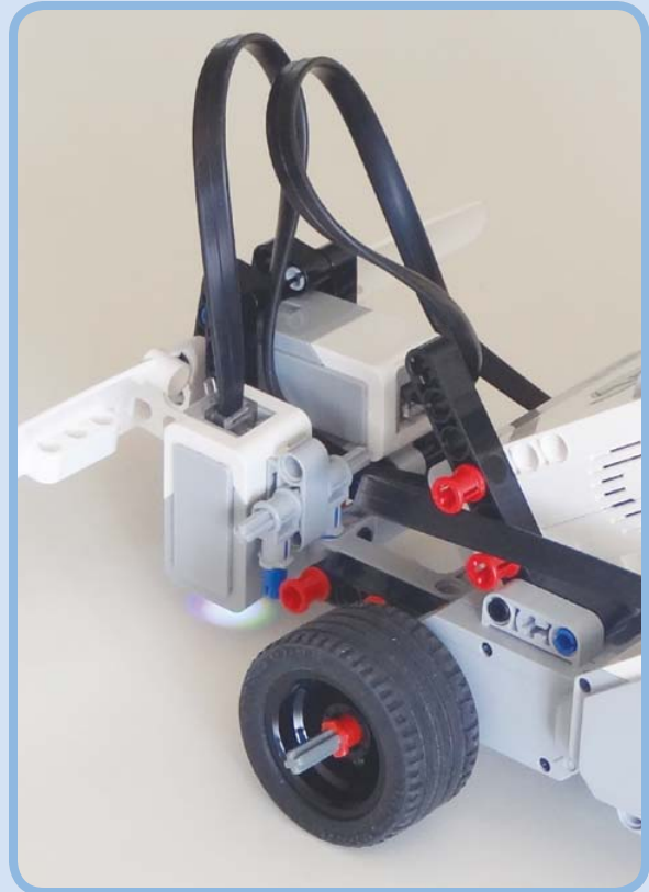
Figure 7-18: The EXPLOR3R with both the Color Sensor (port 3) and the Touch Sensor (port 1) attached. Note that the line-following programs you created earlier should still work with this configuration.
