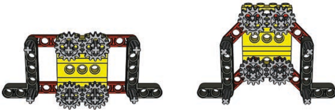
Figure 7-17: Two pairs of parallel levers connected by gears are installed on the element between them. The gears make the pairs rotate in opposite directions, moving the parts at both ends horizontally.
