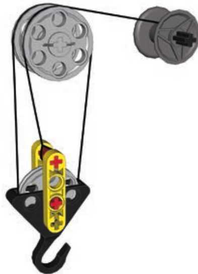
Figure 6-18: A pulley system with three sections of string between the groups. The upper group has string coming through it twice and hence two pulleys to prevent the string from getting tangled up. The string is then tied to the red axle in the lower group. This arrangement grants a mechanical advantage of 3.
