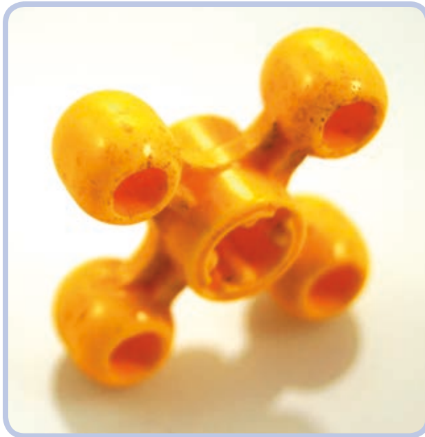
Figure 11-54: This visibly worn knob has polished edges where the material has been rubbed away. Knobs transfer high torque over very small areas of contact, resulting in intense wear. Worn knobs produce a distinctive squeaking when working under stress.
