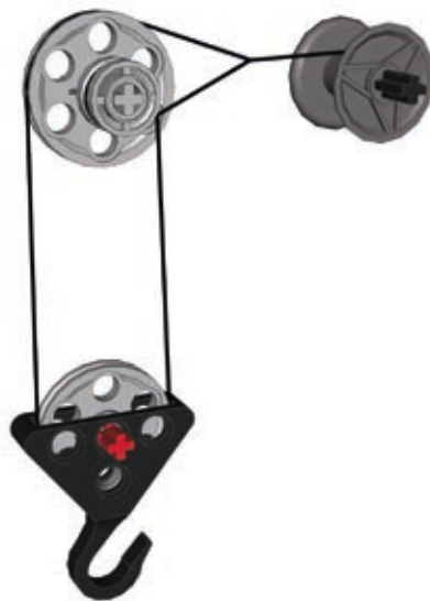
Figure 6-22: Differential block and tackle with two independent pulleys of different diameters in the upper block
