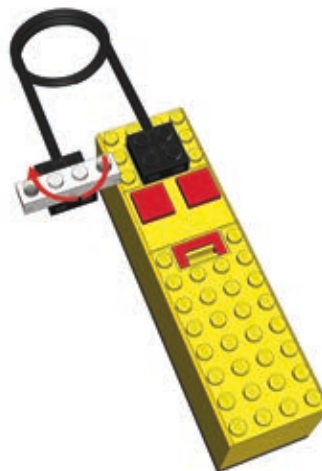
Figure 8-25: A 1×4-stud 9V brick with lights connected to a 9V battery box. By rotating the brick on the plug 180 degrees, we can switch between its lighting modes.
