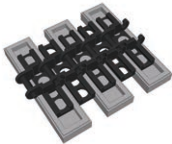
Figure 16-7: A section of older track with tiles added. Note that only every other link can have a piece inserted into it.
