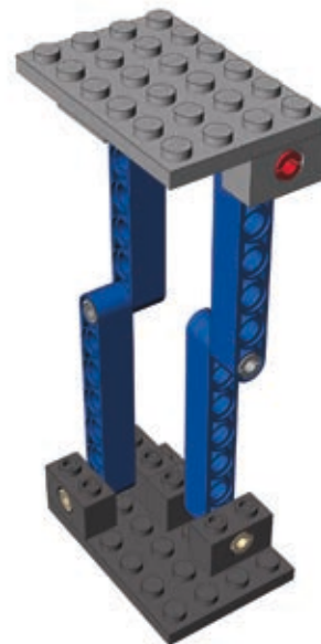
Figure 7-19: The Sarrus linkage's minimum and maximum range of lift
