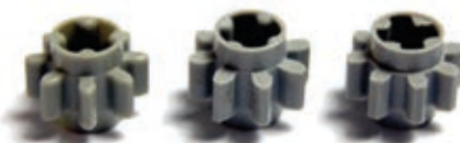
Figure 5-14: Three variants of the 8-tooth gear, from left to right: the initial one, the middle one, and the reinforced one
