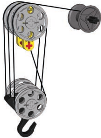
Figure 6-21: This system, called threefold purchase, grants a mechanical advantage of 6.
