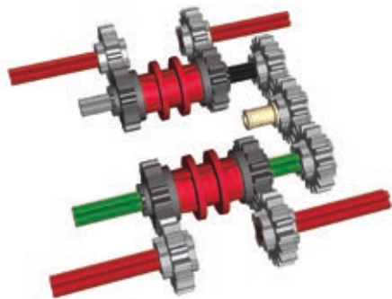
Figure 17-14: A synchronized distribution transmission with four outputs
