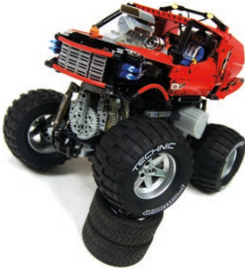
Figure 15-11: My Monster Truck model was a good example of independent suspension. Note that the vertical orientation of both front wheels was identical despite the extreme difference in their heights.
