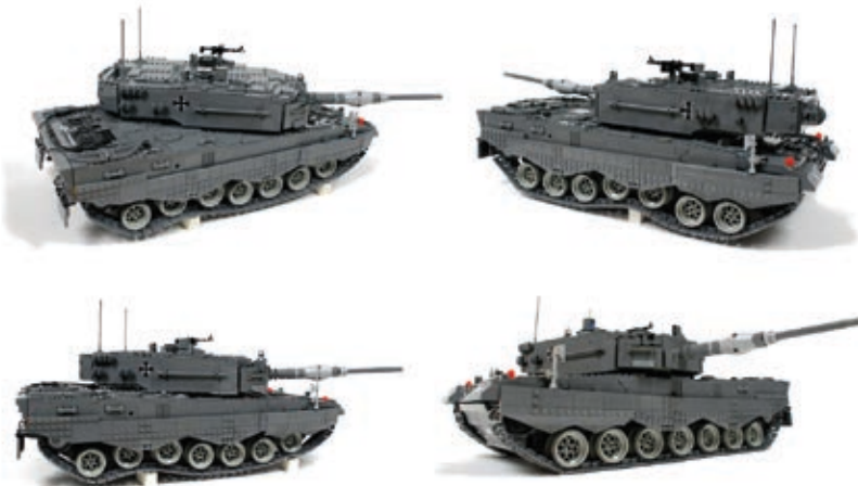
Figure 19-12: My model of the Leopard 2A4 tank was large and heavy. I used four XL motors for propulsion, powered from two battery boxes located in the middle of the hull. It wasn't fast, but it had plenty of torque and handled obstacles extremely well for its weight.
