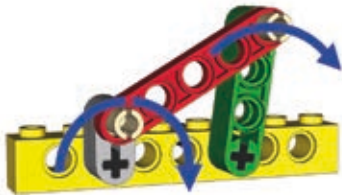
Figure 8-14: An eccentric mechanism with beams instead of discs. Because the second beam (green) makes only a partial rotation, the mechanism takes up less space.
