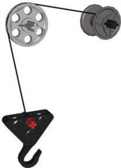
Figure 6-16: This arrangement has an upper group with a single pulley and no lower group. The string that comes off the pulley is tied directly to the hook. No pulley system is created, and no mechanical advantage is gained.
