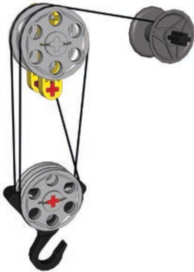
Figure 6-19: This system, called double tackle, grants a mechanical advantage of 4.
