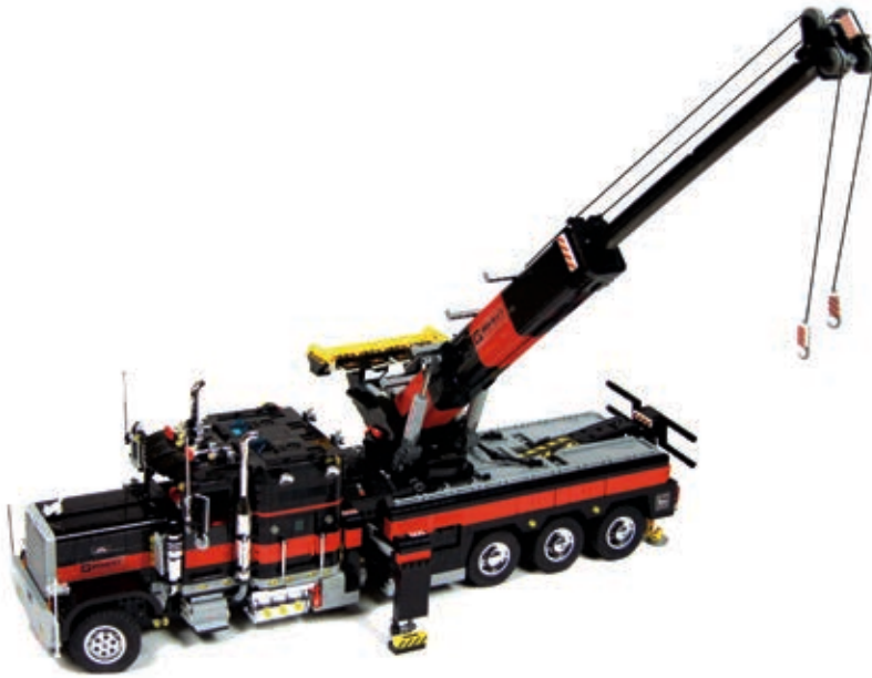
Figure 11-34: My Tow Truck 2 model was very heavy and almost 0.8 m long. It was held together by a massive studfull body frame with two pairs of rails, rigid enough to allow the model to be lifted by hand without any problems. The boom of the truck had its own frame of four studless rails, with the extendable section placed in the middle. It was covered with a studfull shell, which not only made it look better but also improved its rigidity.
