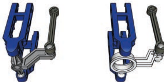
Figure 14-17: Steering arms from the 8865 (left) and 8880 (right) sets, mounted in suspension arms (blue). Both have shifted pivot points to allow Ackermann geometry; the 8880 arm also allows the wheels to be driven.
