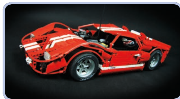
Figure 3-31: My Ford GT40 model used studfull pieces only for minor details of the body and cabin interior. It lacked some rigidity, but it weighed only 2.35 kg while being over 0.5 meter long. It’s the counterexample to Model Team builds.
