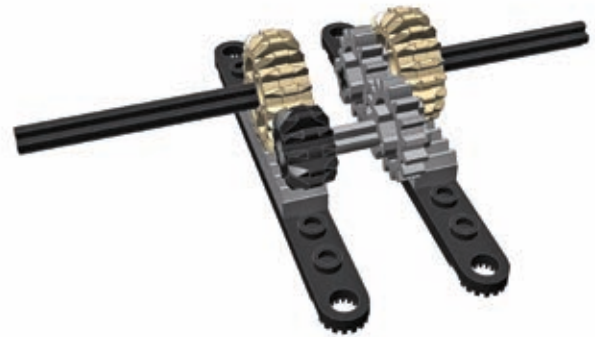
Figure 14-26: Second method for two axles with different steering locks: two identical pinions but two separate steering shafts with gearing between them
