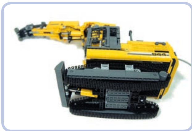
Figure 21-3: My model of the Liebherr R944C tunneling excavator housed more motors in the chassis than it did in the superstructure, at the cost of nearly zero ground clearance. With more space available inside the superstructure, I was able to take better care of its aesthetics.
