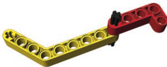
Figure 3-13: When two studless pieces have axle holes, a single axle is enough to create a rigid connection between them. However, such a connection won't be as strong as one made with two or more pins.
