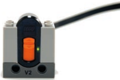
Figure 13-9: The V2 Power Functions receiver. Note the shining indicator LED.
