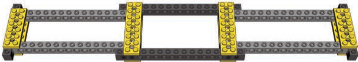
Figure 11-31: A simple studfull chassis combining bricks, pins, and plates
