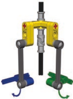
Figure 19-22: A mechanism for tilting a rotor in two planes. Rotating the green axle tilts the rotor in one plane—for example, forward and backward—while rotating the blue axle tilts the rotor in another plane—for example, left and right. Thanks to the use of links and towballs, both angles of the rotor can be changed simultaneously without interference.
