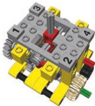
Figure 17-9: The 4-speed synchronized transmission with a single control lever moving in an H pattern. Note the special so-called “changeover plates” (light grey) used to control the shifting lever’s movement and to support the axle it moves along.
