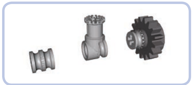
Figure 4-9: Several LEGO pieces can be meshed with a toothed half bush.
