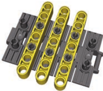
Figure 16-12: Section of the newer track with beams attached
