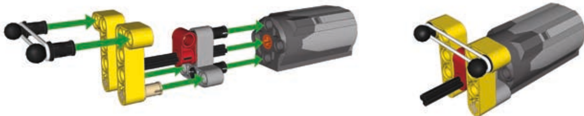
Figure 14-12: The rubber band-based return-to-center steering attachment for a PF Medium motor
