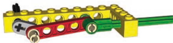
Figure 8-12: An eccentric mechanism with a shorter beam instead of a disc
