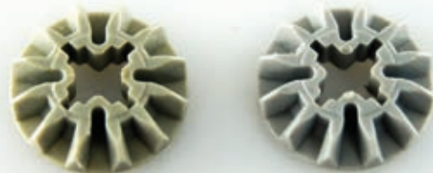
Figure 11-51: Two gears of the same type made roughly 10 years apart
