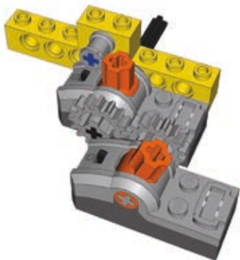
Figure 8-30: Two hard-coupled switches with one of them blocked. The hard-coupling makes the block work on both switches.
