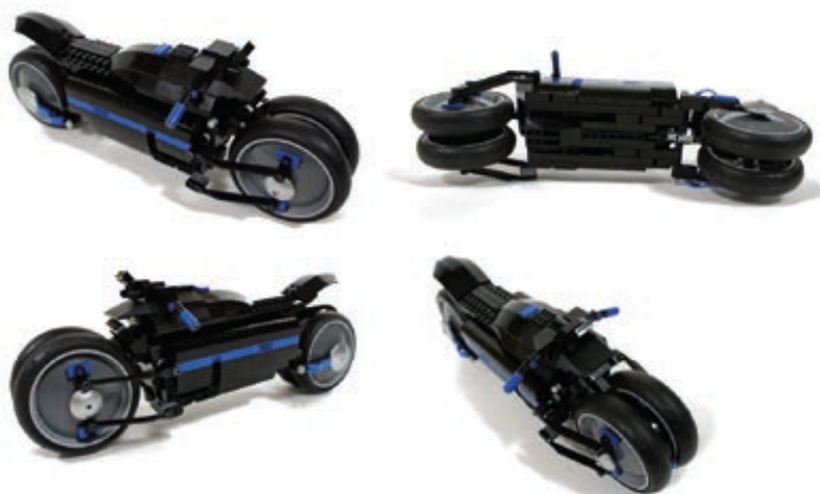
Figure 19-9: The Dodge Tomahawk concept motorcycle comes with double front and rear wheels, thus providing four fulcrums rather than two. I built a motorized model of this bike to prove that it could be motorized and drive stably; however, it couldn't turn because it was too small to house a steering system and a propulsion system at the same time.
