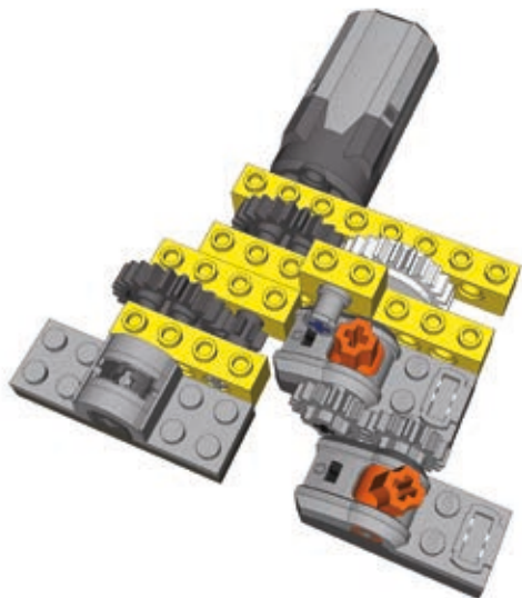
Figure 8-31: Two hard-coupled switches connected to a motorized flashing-light mechanism that uses an old 9V switch. Note the gear down between the motor and the 9V switch—it lowers the flashing rate of the lights to a realistic value.
