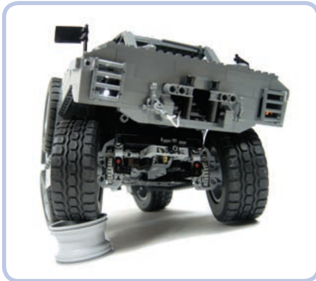
Figure 15-22: My model of the RG-35 4x4 MRAP vehicle made use of LEGO hubs to achieve an impressive ground clearance exceeding 6 studs.
