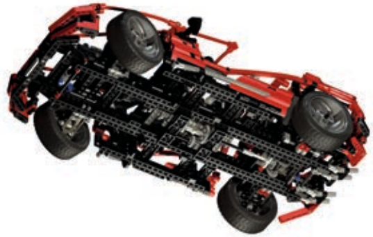
Figure 3-19: The 8448 Super Street Sensation set features a large supercar with a studfull chassis under a studless body. The model combines the rigidity of the studfull pieces, crucial at this size, with the lightness of studless ones.
