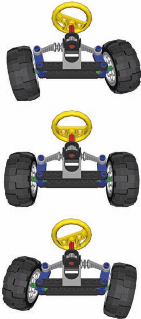
Figure 14-2: Our simple steering mechanism in extreme left, straight, and extreme right positions
