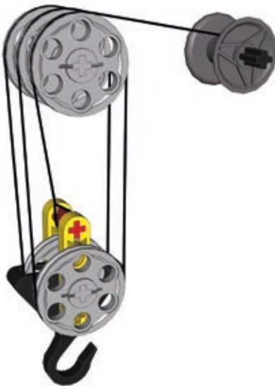
Figure 6-20: This system, called gyn tackle, grants a mechanical advantage of 5.
