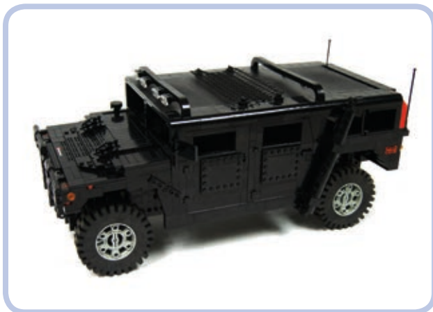
Figure 3-28: My Humvee model used a studfull body on a mixed chassis. The central bearing structure of the chassis was studfull, and the areas between wheels, where compactness was crucial, were studless. The resulting model was very rigid and compact for its functionality but also very heavy.
