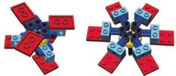
Figure 19-24: A six-bladed hub can be built by doubling the three-bladed version or by simply attaching the blades to a wedge belt wheel with pins so that the centrifugal force of the rotating rotor aligns them.
