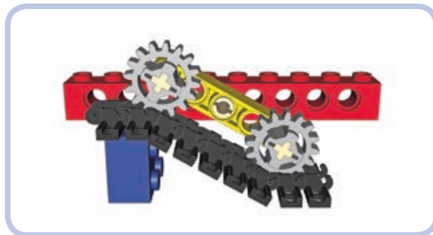
Figure 16-20: In this example, one road wheel is raised by 2 studs, but the bogie's central axle (and thus the vehicle) is raised only by 1 stud.
