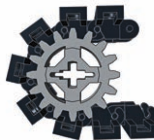
Figure 16-6: A section of older track wrapped around a 16-tooth gear
