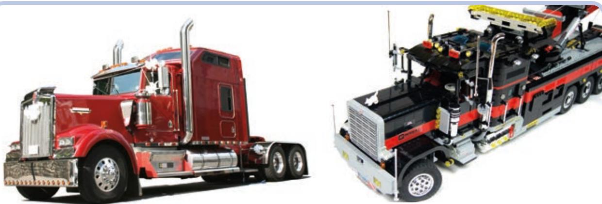
Figure 21-13: Because of their unrealistic steering geometry, LEGO wheels need more spacious mudguards than real wheels do. If the mudguards of my tow truck weren't sized up relative to the real ones, the wheels would collide with them.
