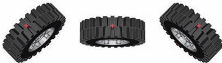
Figure 21-9: The steering geometry of a real vehicle's wheel: As the wheel is steered, it rotates around a pivot point going through its center, marked in this series of images by an "imaginary" red axle.
