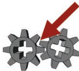
Figure 1-3: Backlash, in the form of a gap between the teeth of two mating gears, is particularly large for 8-tooth gears.
