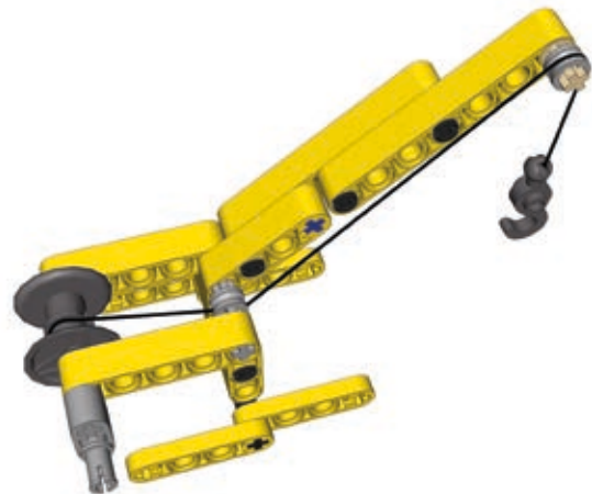
Figure 6-14: A simple crane uses a winch to pull a load on a hook up and down. The movement is transferred through a string, which is guided from the reel to the top of the crane by two half bushes acting as idler pulleys.
