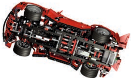
Figure 3-21: The 8070 Super Car set can be considered a direct descendant of the 8448 set. It's completely studless, with a very rigid, although shorter, chassis.
