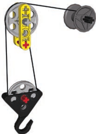
Figure 6-17: This arrangement has two groups, each with a single pulley. The string comes off the upper pulley and around the lower pulley and is then tied to the element that is part of the upper group and remains fixed to it. It's the simplest pulley system, with a mechanical advantage of 2.
