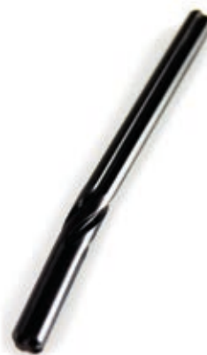
Figure 11-17: Axles are much more elastic than they might seem. This one has been twisted permanently by a PF XL motor.
