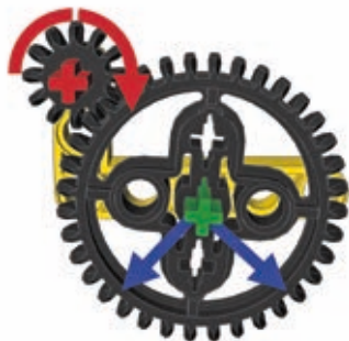
Figure 11-9: The directions of force exerted on the follower gear, which is located below and to the side of the driver gear
