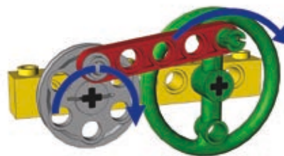
Figure 8-13: An eccentric mechanism with two discs connected by a beam. The smaller disc makes full rotations, and the larger disc makes only partial rotations back and forth.
