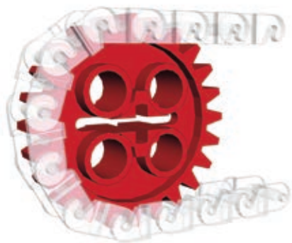
Figure 6-7: A close-up view of the chain wrapped around a gear shows that each link occupies two teeth. The section of the chain that has contact with the gear has no play in it, and its elasticity is minimized.
