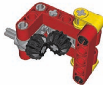
Figure 11-22: Perpendicular gears reinforced with L-shaped beams. Note that one end of the beams is held together by a vertical beam. This is because there are only axles on this end of the beams and the axles don't hold the beams together. The other end of the beams has a connector with pins that hold the beams together with a force very unlikely to be overcome by gears.
