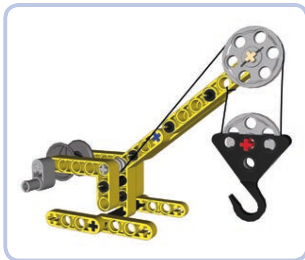
Figure 6-15: Our simple crane equipped with a pulley system. Two groups of pulleys are used, each consisting of a single pulley: The upper one stays on top of the crane, and the lower one moves up and down with the hook. This particular arrangement of string between the pulleys grants a mechanical advantage of 2.
