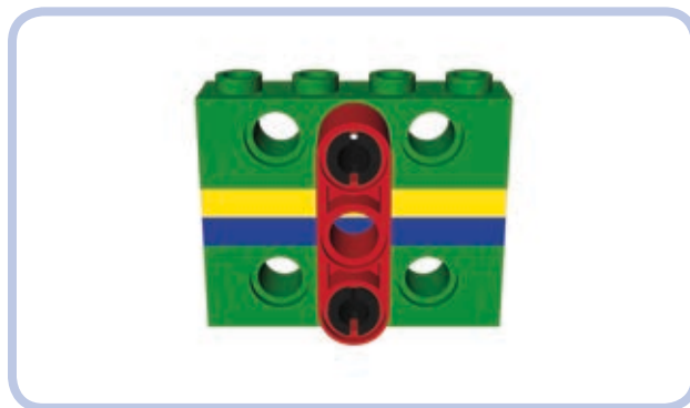
Figure 2-16: The basic rule of alignment for studless and studded pieces: Holes in two bricks separated by two plates are exactly 3 studs apart.
