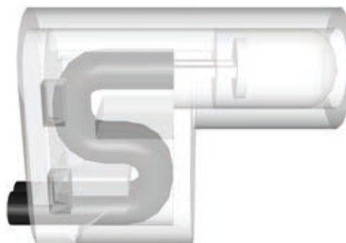
Figure 13-21: Side view of the LEGO LED. You can see part of the wire tucked in to prevent it from being ripped off. The actual LED is located in a protruding tube that fits into a pin hole and is slightly less than a single stud long.
