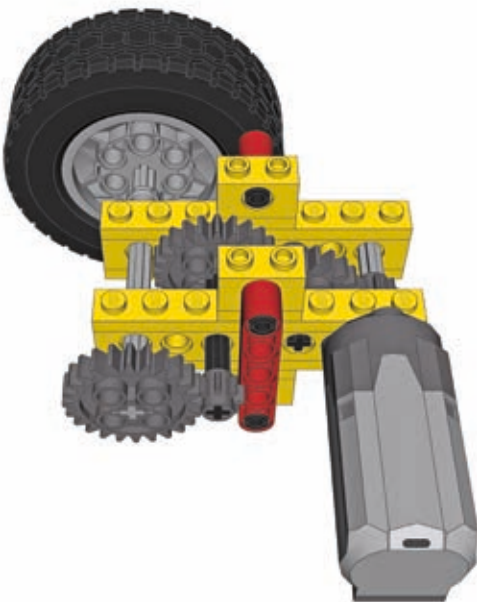
Figure 11-6: Vertical beams (red) are a popular means of reinforcement.
