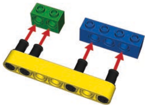
Figure 3-32: Beams can be easily connected with bricks using pins. Note that we can choose regular Technic bricks (blue) or bricks with centered pin holes (green) to adjust the alignment.
