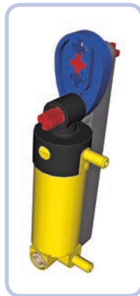
Figure 10-16: To make the cylinder extend fully, we need its tip to be mounted 1.5 studs away from the shaft. A piece called a Technic cam allows this.
