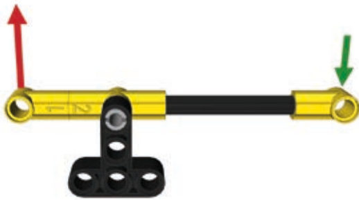
Figure 7-5: Class 1 lever with the fulcrum in the middle and the effort (green) and load (red) at its ends
