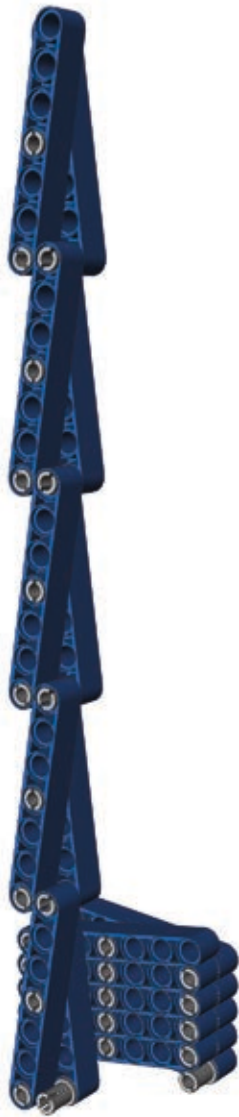
Figure 7-21: A comparison of the same 10-link-long scissor linkage in a fully retracted and a fully extended position
