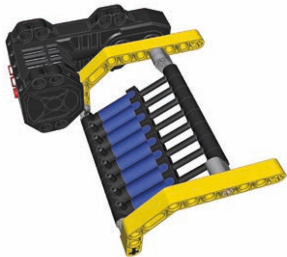
Figure 10-1: An eight-pump compressor driven by the RC motor. This design is a real monstrosity in the world of LEGO compressors.
