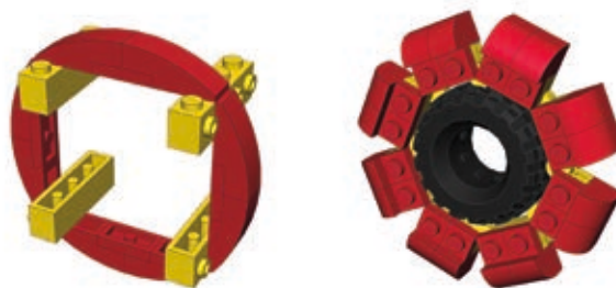
Figure 21-15: Two circular structures built with small basic pieces. One is built around bricks with studs on the side, and the second is built with hinge plates embracing a tire. Both are prone to disintegration if sufficient stress is applied.
