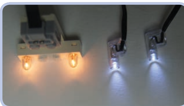
Figure 8-26: A 1×4-stud 9V brick with lights (left) and a pair of Power Functions LED lights (right). Note the difference in the color and direction of the light.
