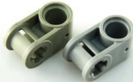
Figure 11-50: A connector: old (left) and new (right). Even though the old piece is free from damage or visible wear, the difference is obvious.
