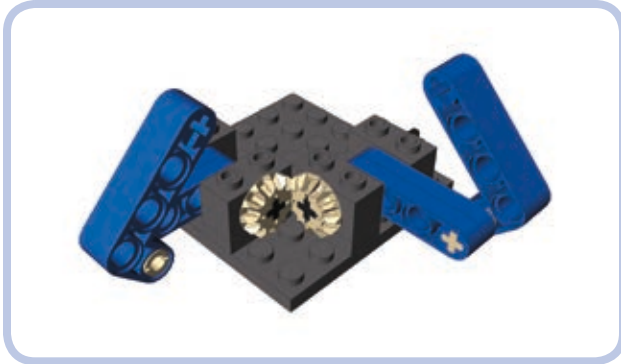
Figure 7-20: This Sarrus linkage uses mated bevel gears to synchronize links between the two groups.
