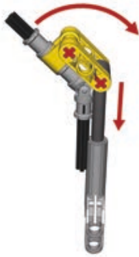
Figure 19-21: An example of a simple rotor-tilting mechanism. The black axles with a universal joint are the driveshaft, connecting the rotor on the top with a motor on the bottom. Retracting and extending the linear actuator changes the angle of the axle above the joint and thus of the whole rotor.
