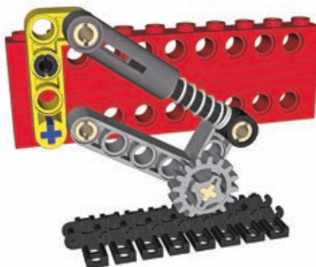
Figure 16-22: A simple trailing arm with a shock absorber
