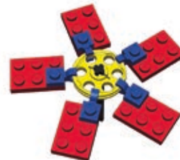
Figure 19-25: Finally, a hub with any number of blades can be built by attaching 1x1 plates with clips to the edge of a wedge belt wheel. This solution, invented by Polish builder Marcin “Mrutek” Rutkowski, results in a surprisingly robust setup, which can be made even stronger if you attach blades using two wedge belt wheels and two clips. You will, however, need to align the blades by hand, so a protractor may be useful.
