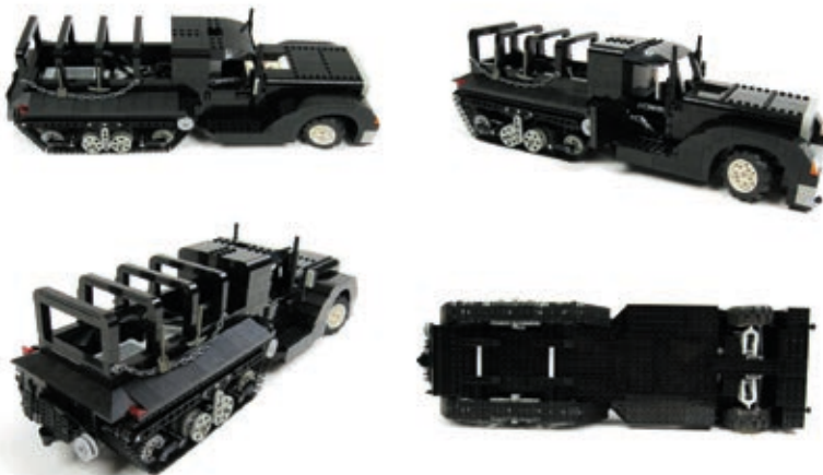
Figure 19-13: My model of a half-track truck. Vehicles of this type are driven by tracks and steered by front wheels.
