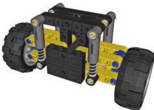
Figure 15-10: Independent suspension with four shock absorbers supporting the chassis against the suspension arms
