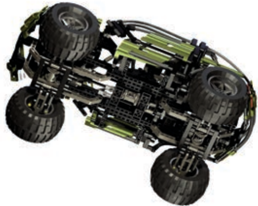
Figure 3-20: The 8466 4x4 Off-Roader set features another large car model, but this time only the center of the chassis remains studfull. This center provides the rigidity needed by the car's impressive suspension system, but the set itself is mainly studless.
