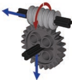
Figure 11-26: The directions of forces exerted by a worm gear. Unlike regular gears, a worm gear doesn't push the follower gear to the side; instead, it pushes itself against the follower gear along its axle.
