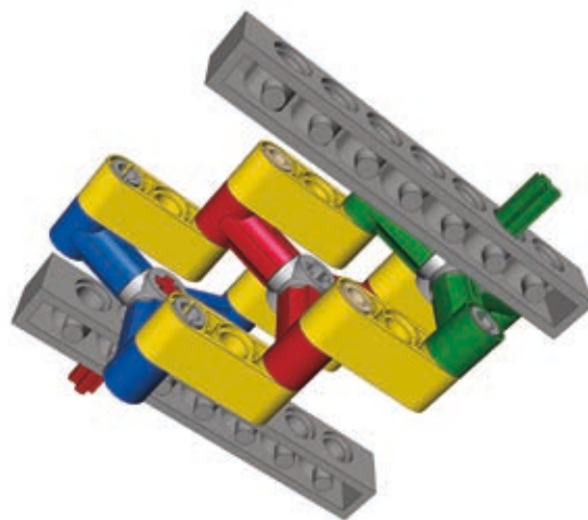
Figure 8-19: A Schmidt coupling with three triangles (in green, red, and blue) and six links (yellow). Note that the middle triangle (red) doesn't need any support—it can even move as the coupling works.
