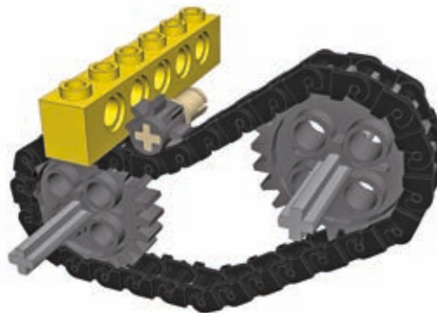
Figure 6-6: The 8-tooth gear also works with a chain but cannot drive it due to its small size. It can still be used as an idler gear, adapting the shape of the chain to the surrounding structure.
