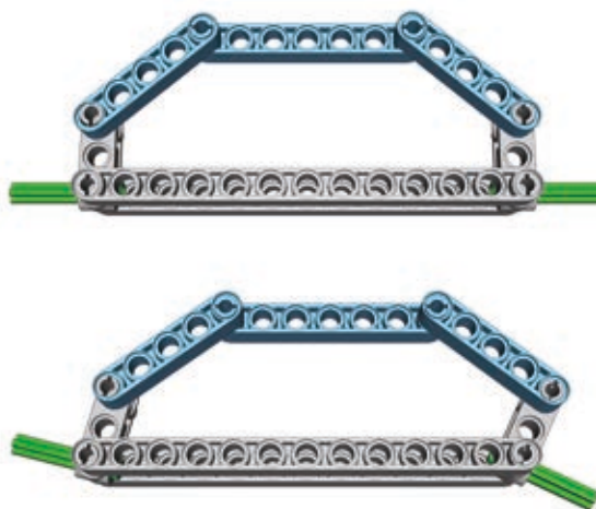
Figure 14-18: Ackermann steering geometry achieved by using a three-piece tie rod with a longer central section
