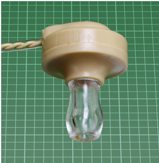
Figure 29-8. A vintage earphone of the type suitable for use with a crystal-set radio.
