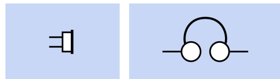
Figure 29-1. Schematic symbols for a single earphone or headphone (left) and a pair of headphones (right).
