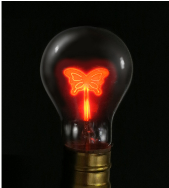
Figure 19-10. In bygone decades, ornamental neon bulbs with specially shaped electrodes were popular.
